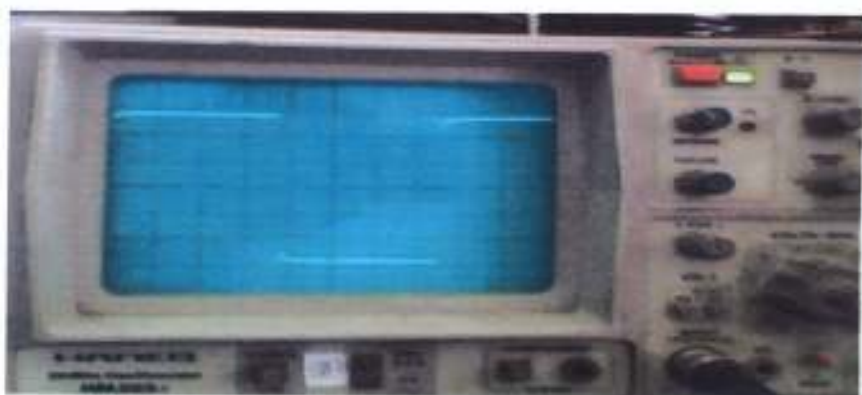
Fig. 3.17 Photographs of the Oscilloscope display of the inverter oscillator output Waveform for different time base settings
