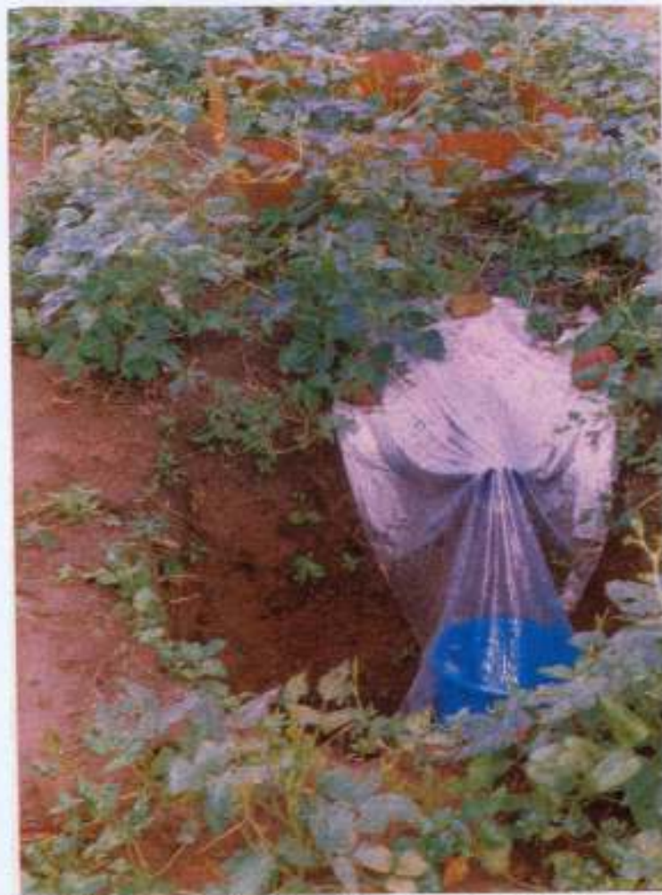
Plate 2B A view of the Runoff metre Installation on field
