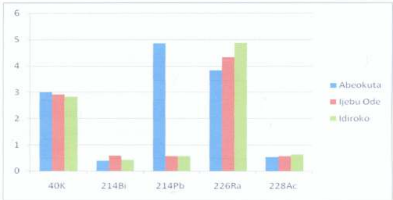
Figure 4.3: Bar Chart showing the activity concentrations (Bq l -1 ) of 40 K, 214 Bi, 214 Pb, 226 Ra and 228 Ac in the three selected cities
