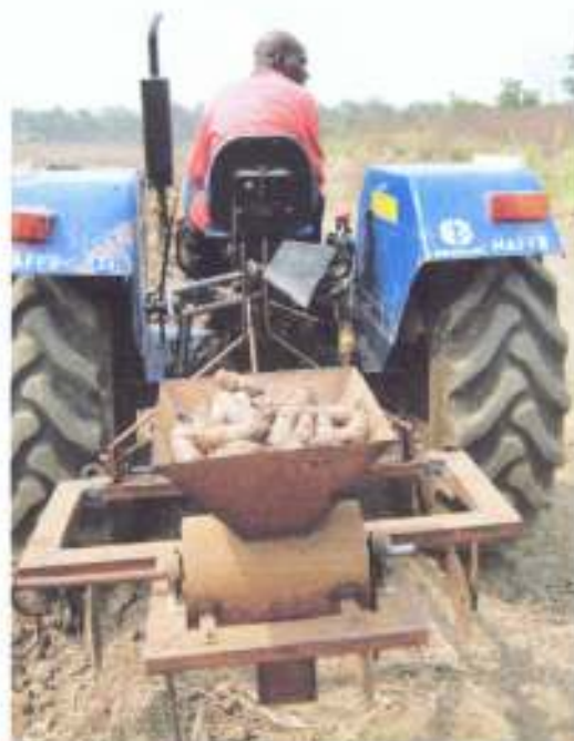
Fig: 4.1: Developed cocoyam planter mounted on a tractor
