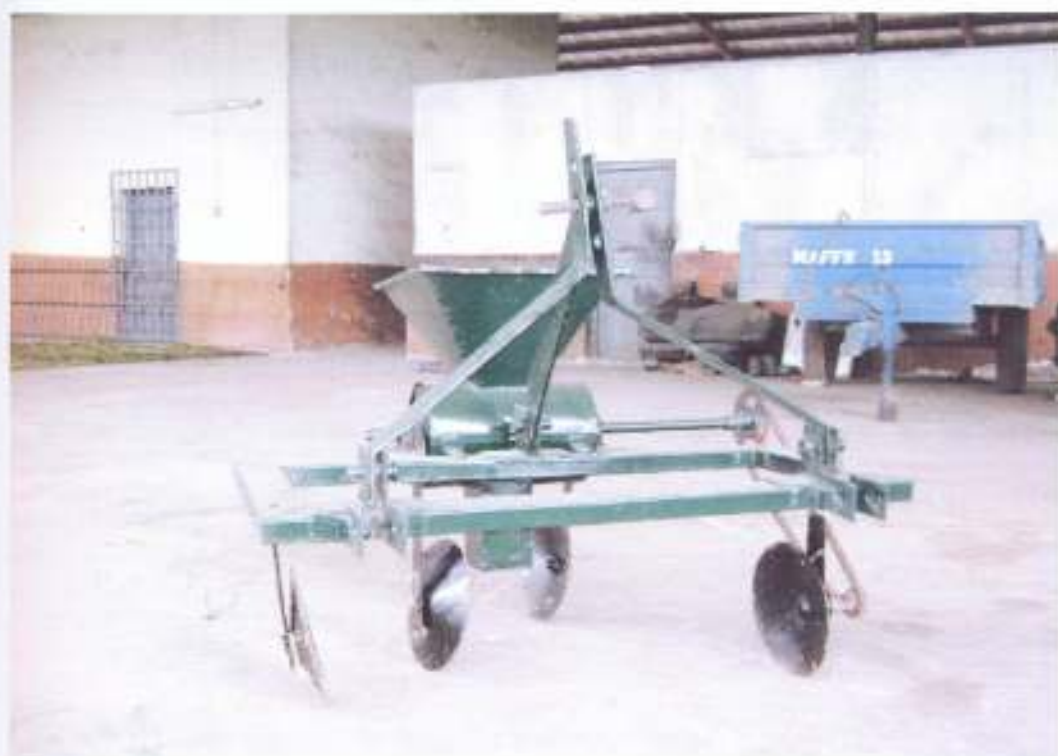
Fig. 3.1: Developed Cocoyam Planter.
