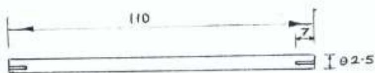
Fig. 34. Schematic Diagram of Stripper Shaft.
