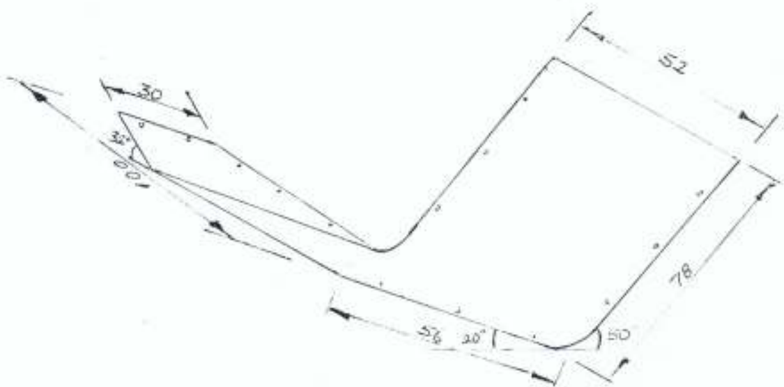
Fig. 26. Schematic Diagram of Stripper Pan.
