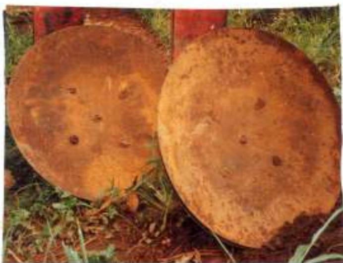
Figure 12 - The deeply corroded, (rough) blade surface.
