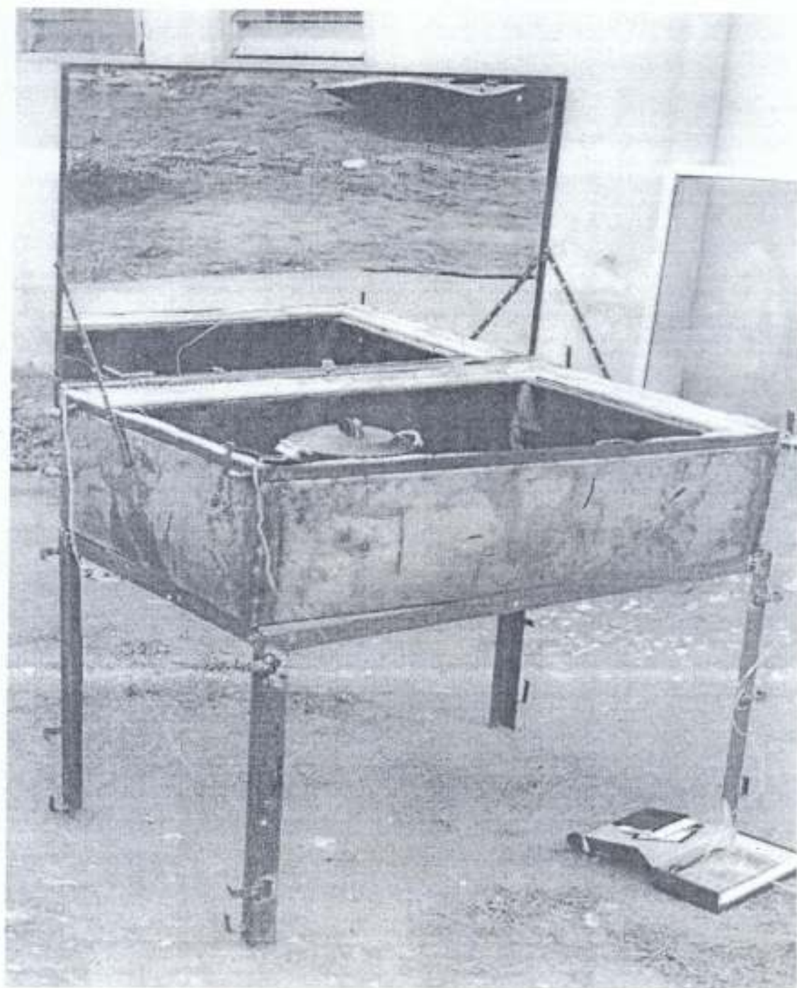
Fig 3.14a The Solar Energy Hot-Box Cooker With a Reflector
