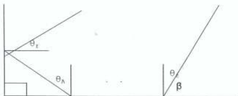
Fig. 3.4: Angle of Incidence of Reflected beam on Glass surface.
