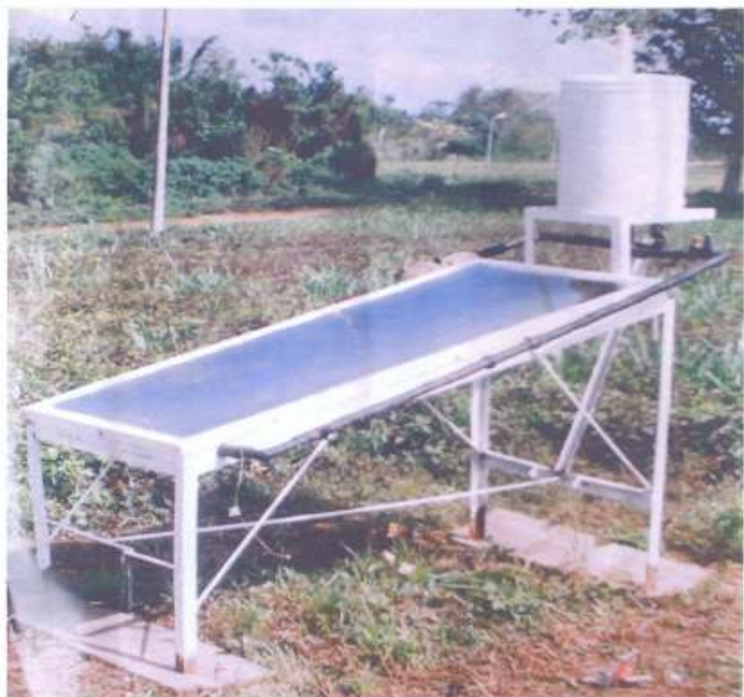
Fig.3.12. Photograph of the locally constructed solar water heater.
