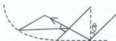
(b) Tracking the sun when its incidence angle is \theta Figs.1.1 Tracking character of Fresnel reflectors
