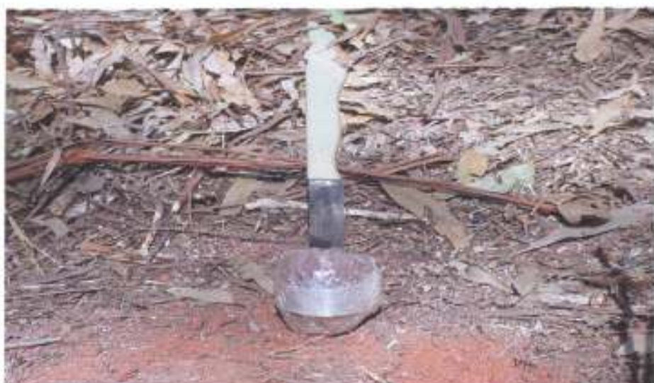
Plate 3.3: Soil Sample Wrapped in Paraffin Wax.
