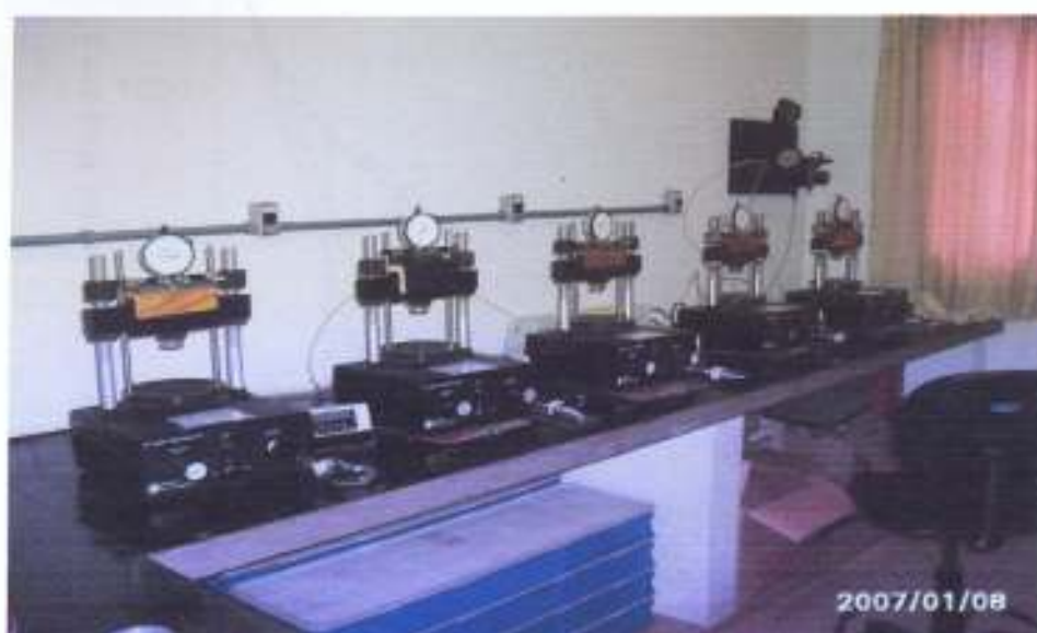
Plate 3.7: Multi Step Consolidometer
