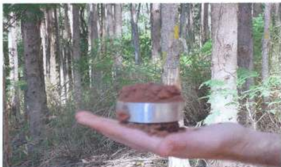
Plate 3.2: Undisturbed Soil Sample in Cylindrical Metal Ring.
