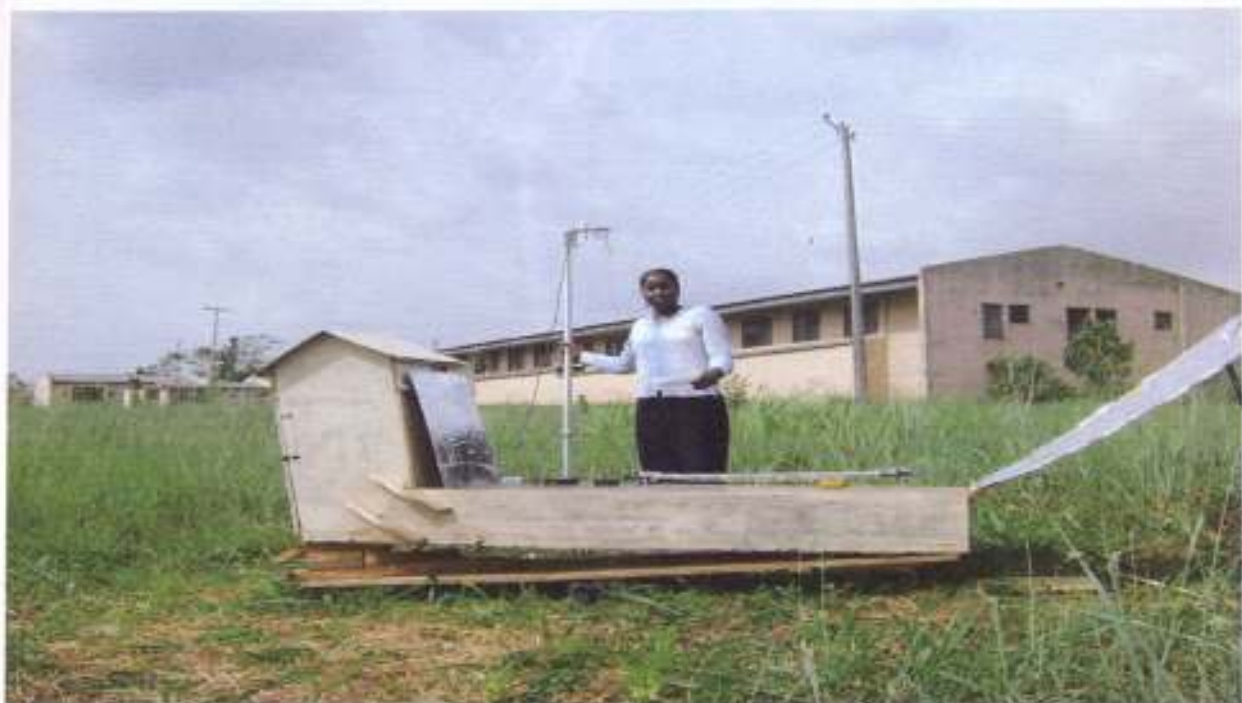
Plate 8 Drying with indirect Solar dryer
