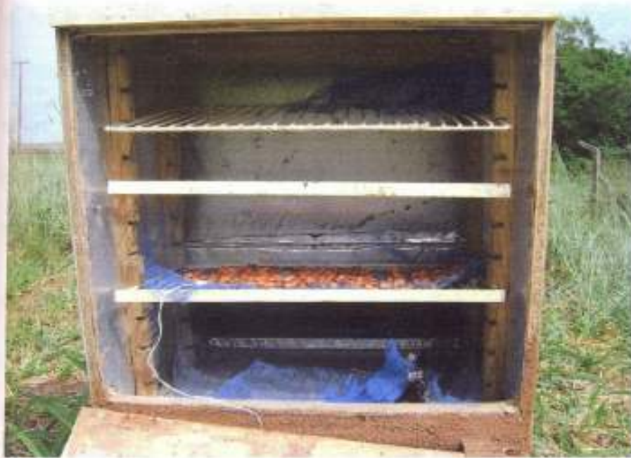
Plate 7 The Drying Chamber and the drying trays
