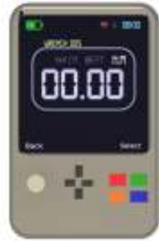
Figure 24: Monitoring System for the Torqueing of Bolts and Nuts on a Telecommunication Mast
