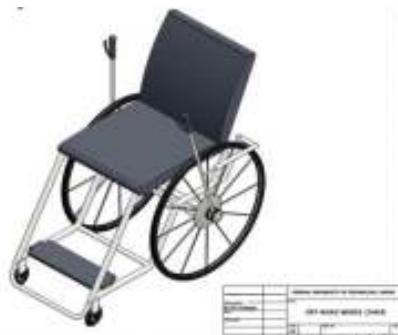
Figure 6: Off-road push-crank wheelchair
