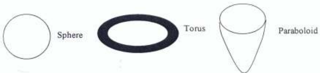
Fig. 171. Double Curved Geometrical Surfaces
