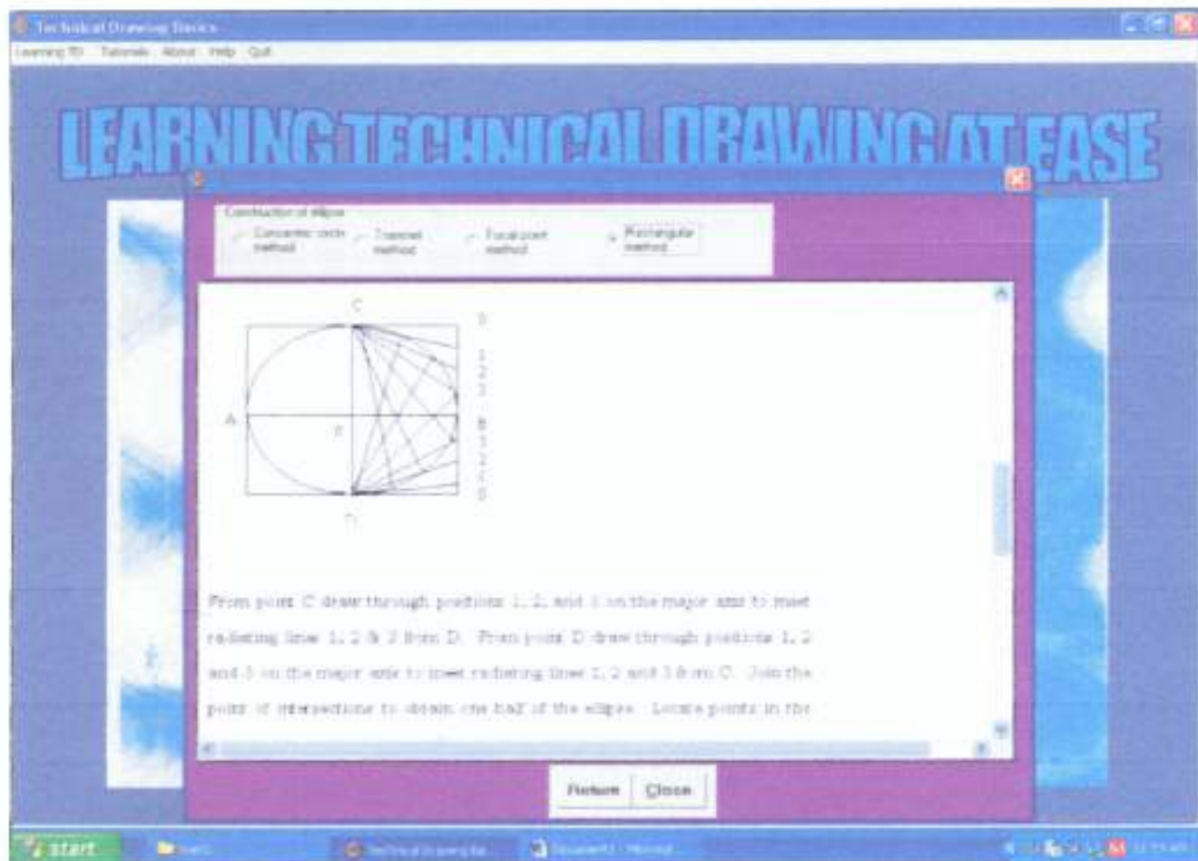
Fig. 4.5b : Learning window giving information about construction of ellipse using the rectangular method
