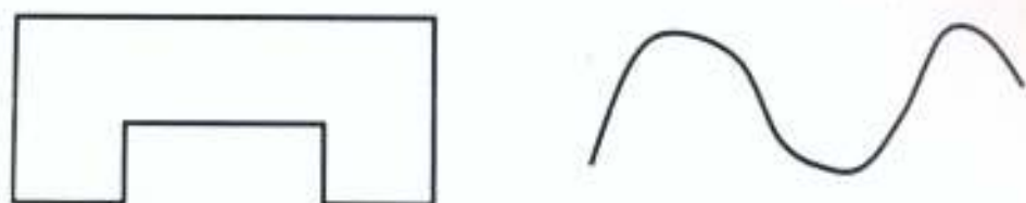
Figure 21c: Complete sketch made by using dots or dashes as guides
