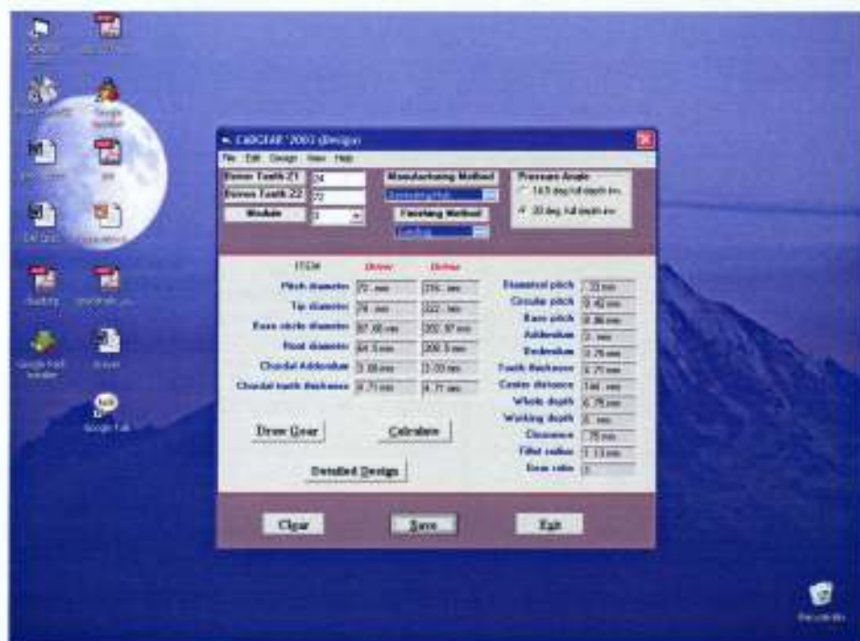
Chart 4.1: Case One Screen Output for Spur Gear Geometric Parameters
