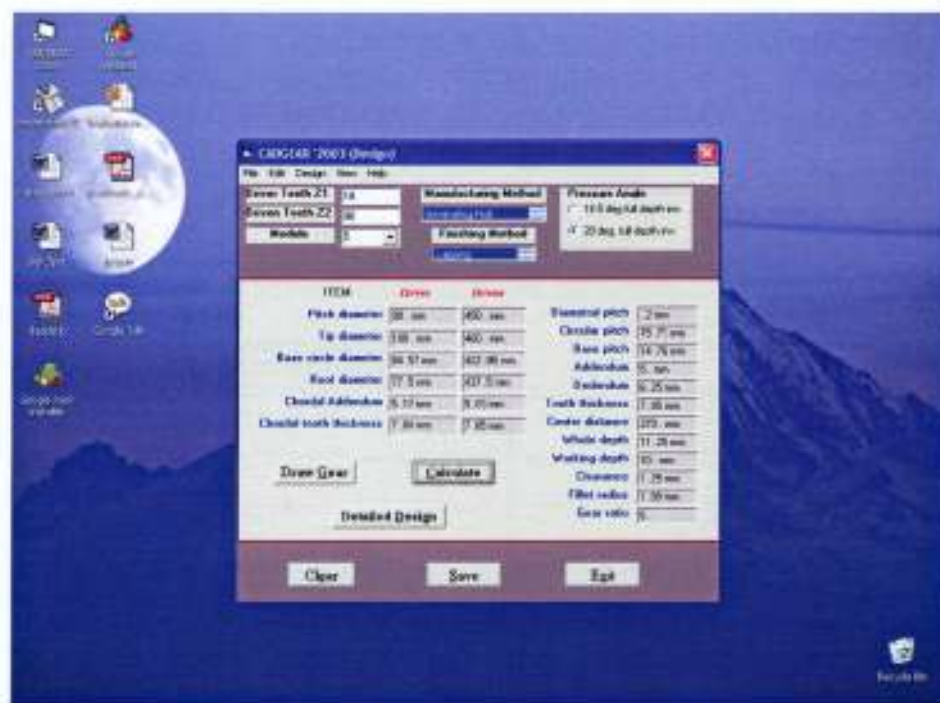
Chart 4.5: Case Two Screen Output for Spur Gear Geometric Parameters
