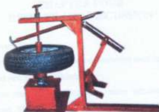
Figure 19: Tyre Fixing Operation
