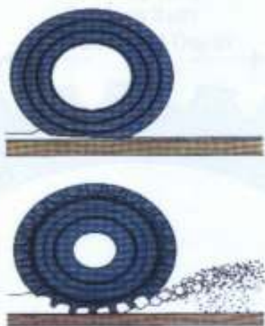
Figure 8: View of Hydroplaning effect on Tyre Source: Readers Digest Association (1981)
