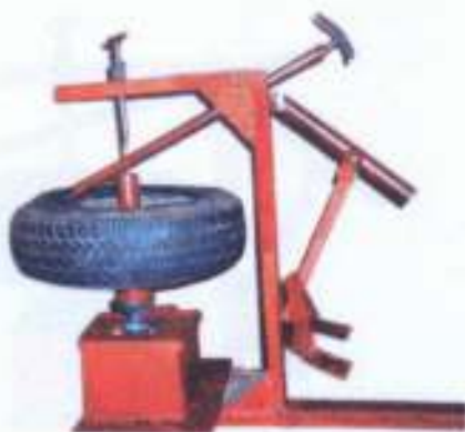
Figure 18: Tyre Removing Operation
