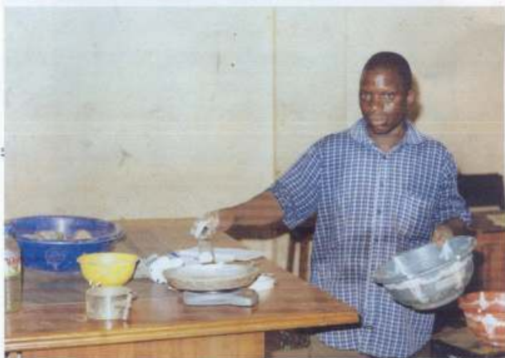
Plate 7: Compacted samples being weighed before testing at the Federal University of Technology Geotechnical Laboratory, Akure.
