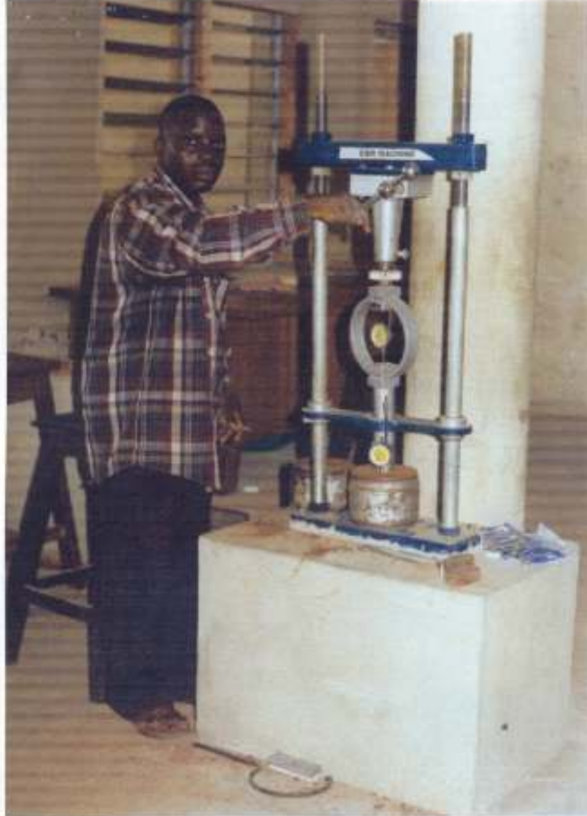
Plate 9: California bearing ratio test being performed on the samples at the Federal University of Technology, Geotechnical Laboratory Akure.
