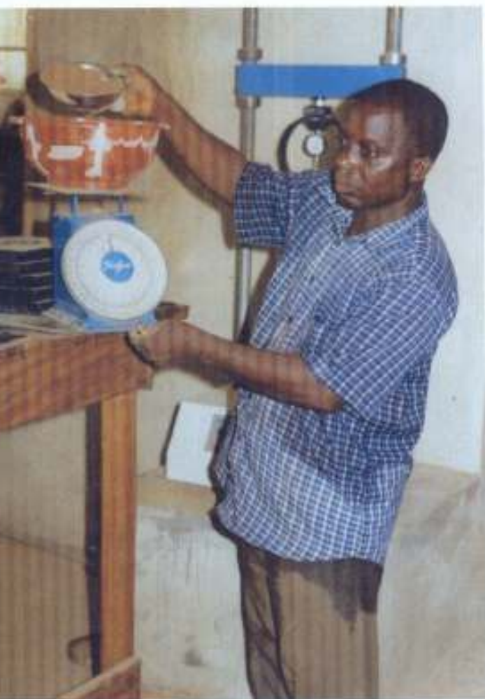
Soil sample being weighed before compaction at the F.U.T.A (Geotechnical Laboratory)
