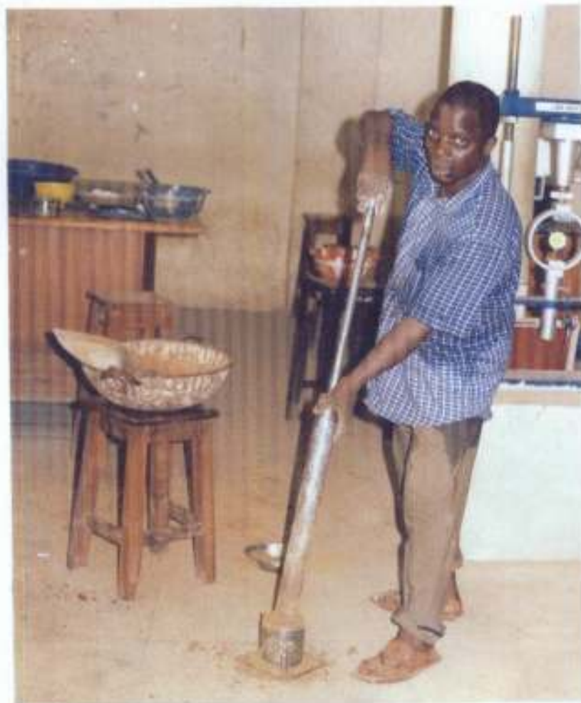
Plate 6: Compaction Test being performed on the samples at the Federal University of Technology Geotechnical Laboratory, Akure.
