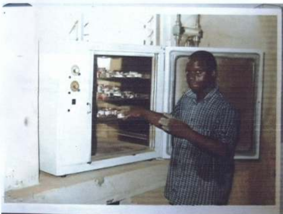
Plate 8: Compacted samples being taken into the oven for drying at the Federal University of Technology Geotechnical Laboratory, Akure.
