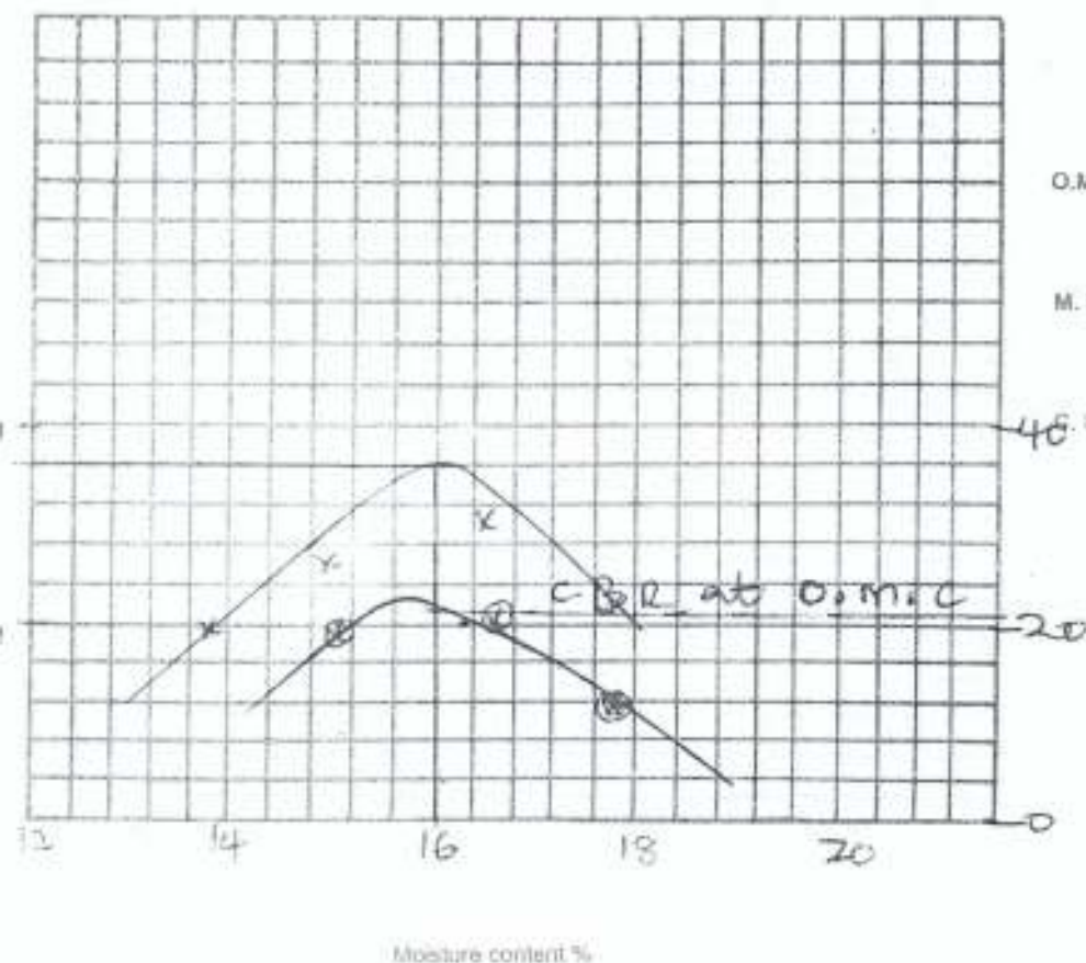
Fig. 2 : Moisture - Density - CBR Relations
