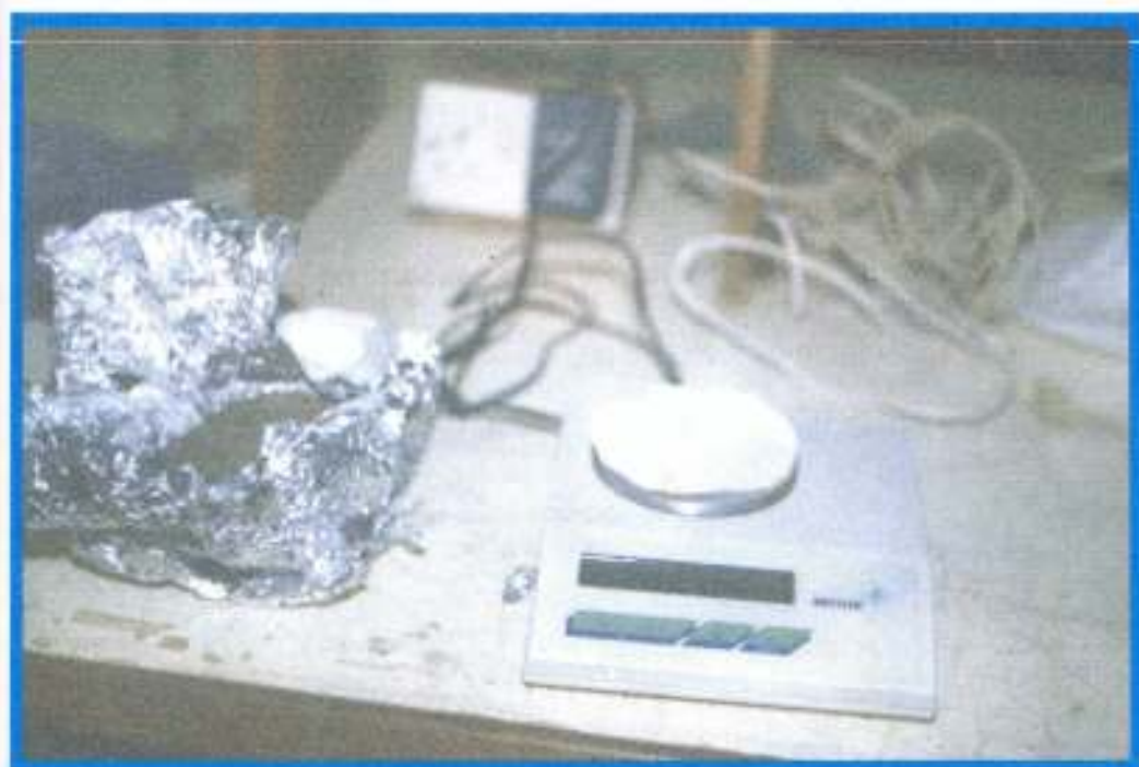
Photo 4.41 (b): Mettler balance for weighing both soil samples and filter papers
