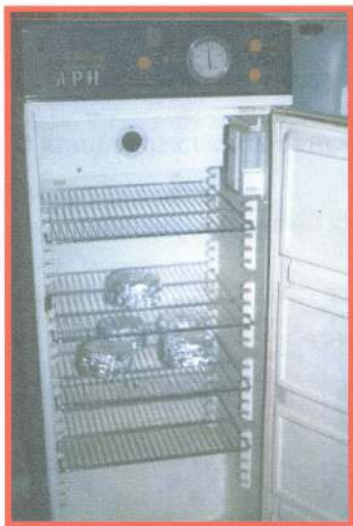
Photo 4.41 (a): Cooled incubator for maintaining constant temperature for one week
