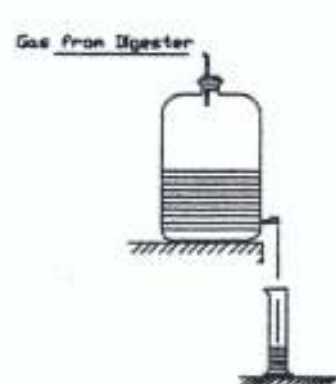
Fig 2.9. Gas collection method using displaced water
