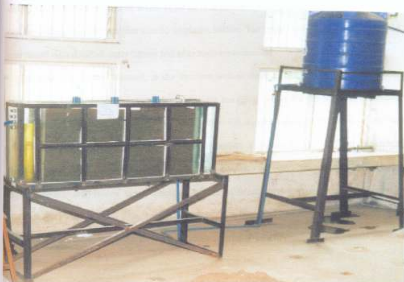
Plate 3.1: Reinforcing Cage for Glass-Perspex Laboratory Sand Tank and the Elevated Water Reservoir.
