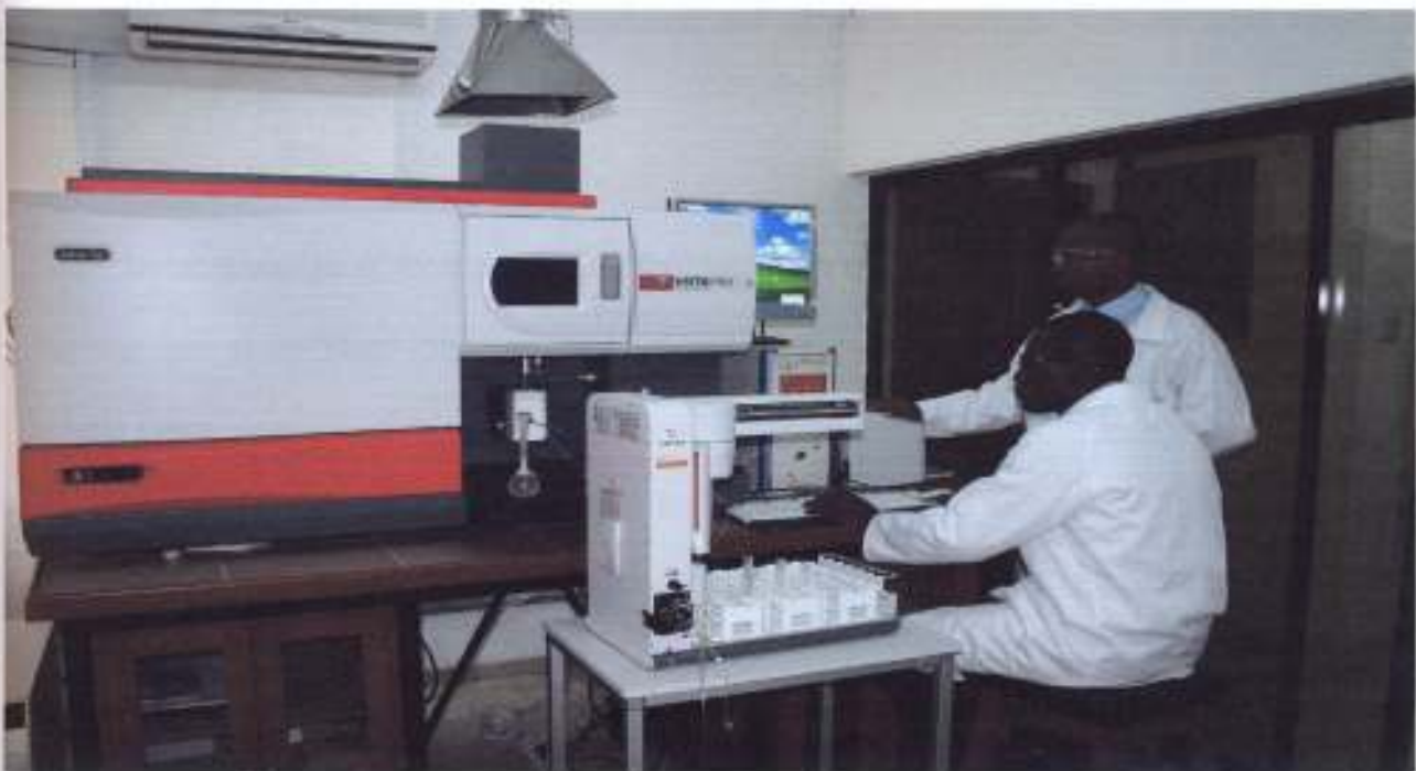
Plate 3.2: Inductively Coupled Plasma Emission Spectrometry for Metal Analysis (Multi-Environmental Laboratory, Ketu, Lagos)
