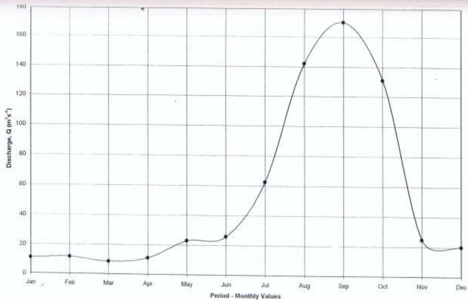
Fig. 5.2 Flow Discharge Hydrograph for Ogbese river (1989 - 1999)
