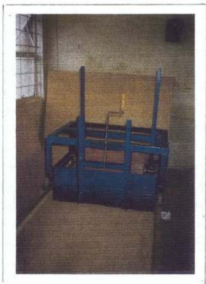
Fig. 40 : The processing trolley, compaction roller and levelling board
