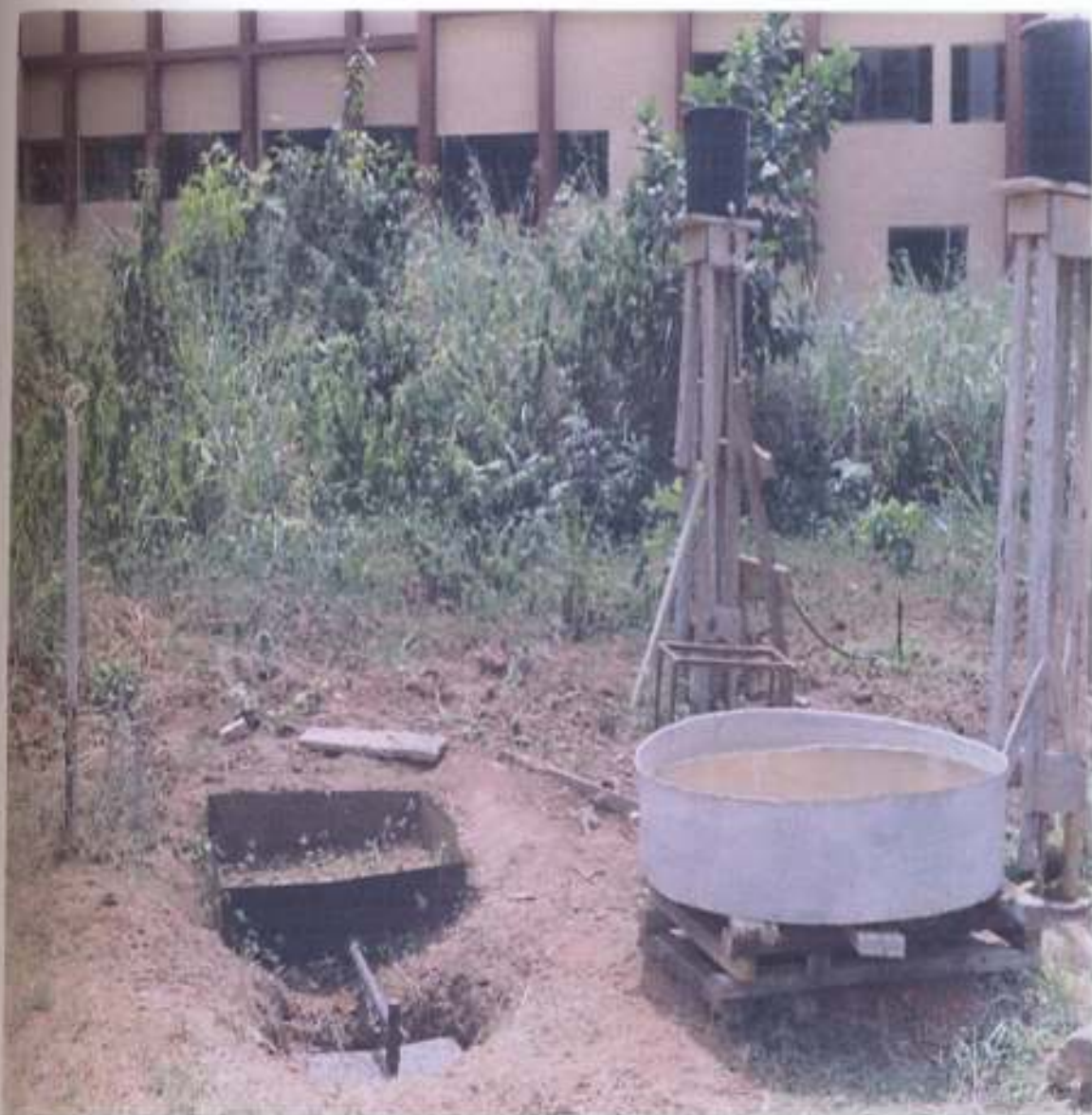
PLATE 2. Field Arrangements of Tensiometer, Runoff Meter and Pan Evaporimeter
