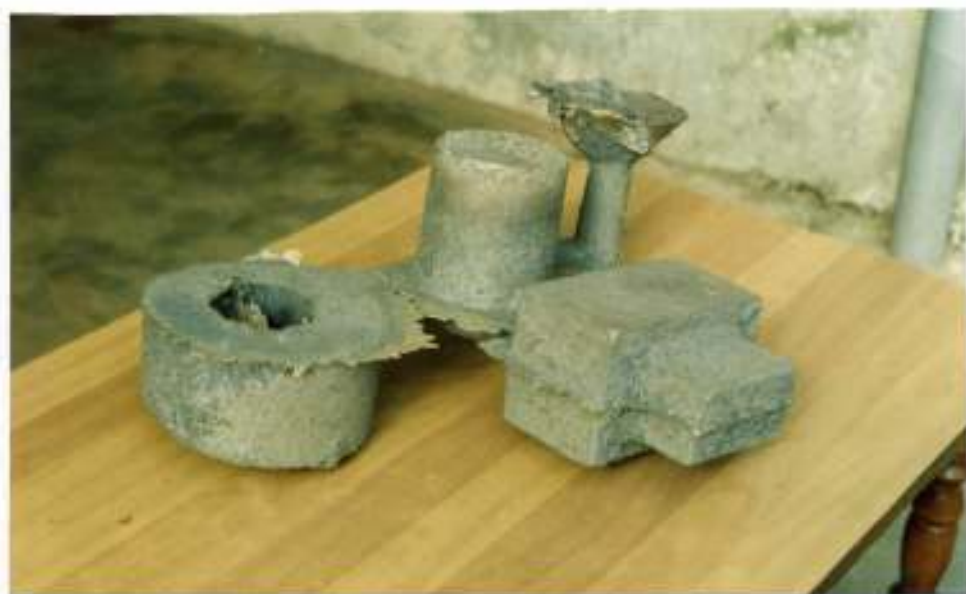
Plate 4.8: Completed Brass Casting
