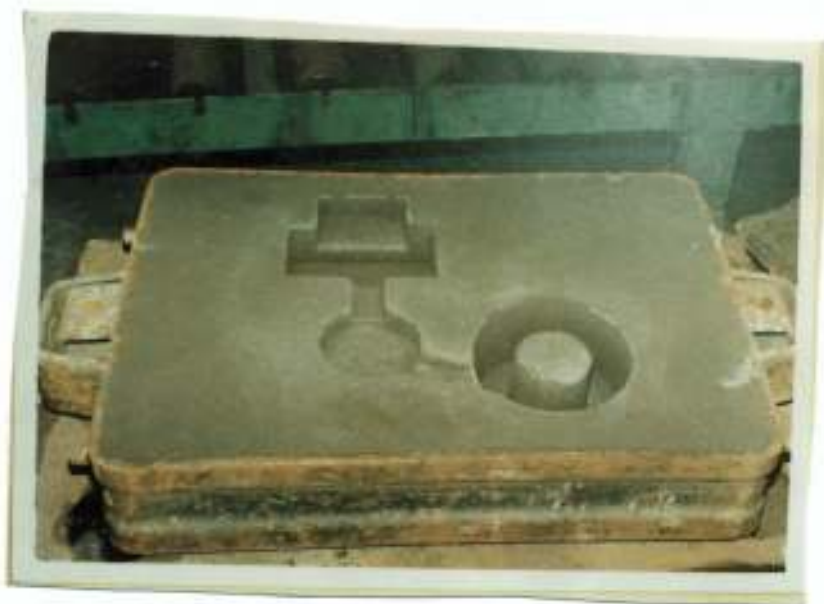
Plate 4.4: Bottom Moulding Box filled up with sand and pattern impression
