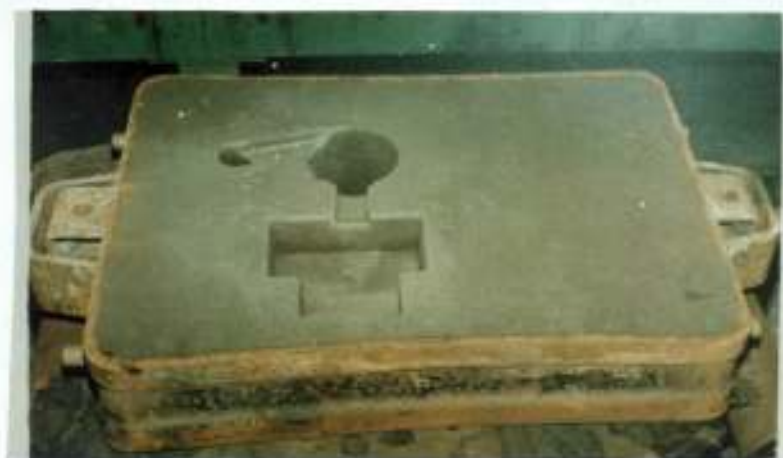
Plate 4.3: The Top Moulding Box filled up with sand and pattern impression
