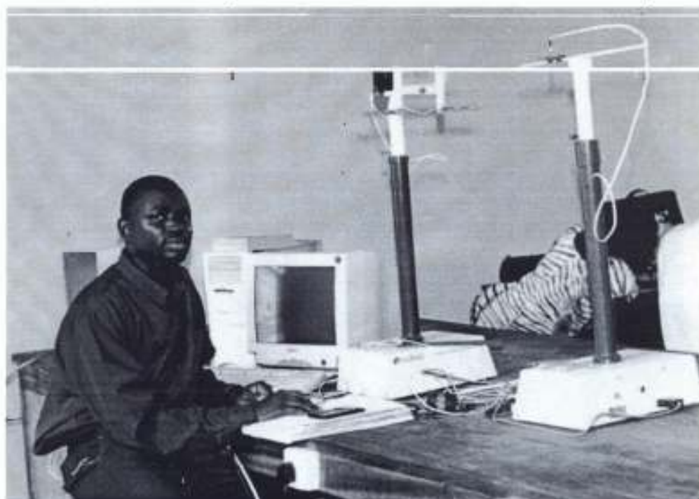
PLATE 3J SETTING UP THE 'ANTENNALAB' SYSTEM FOR THE HARDWARE MODELLING (THE TWO POLES ARE THE GENERATOR TOWER AND THE RECEIVER TOWER)
