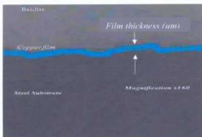
Figure C8: Micrographic view of cross section through copper-steel plating (magnification x160)
