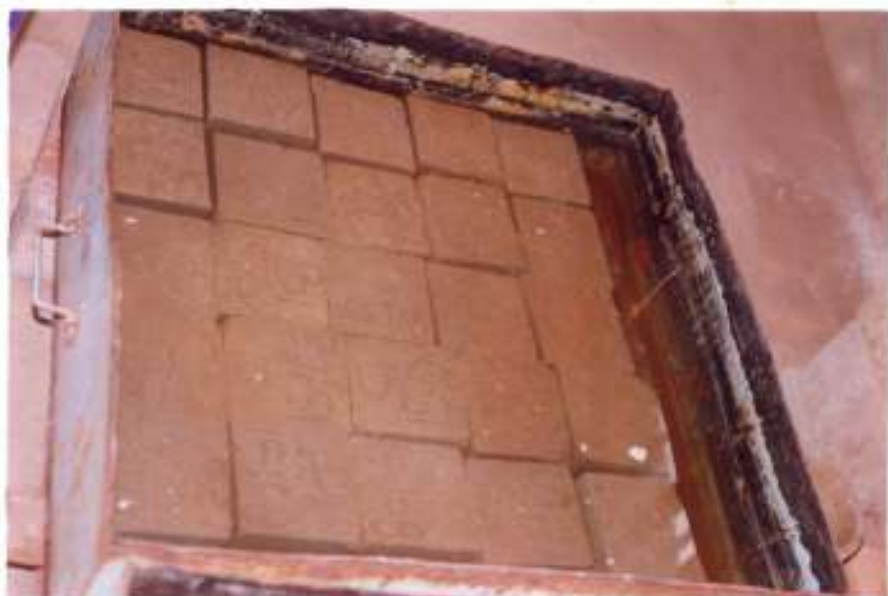
Plate 2 showing cube samples during curing
