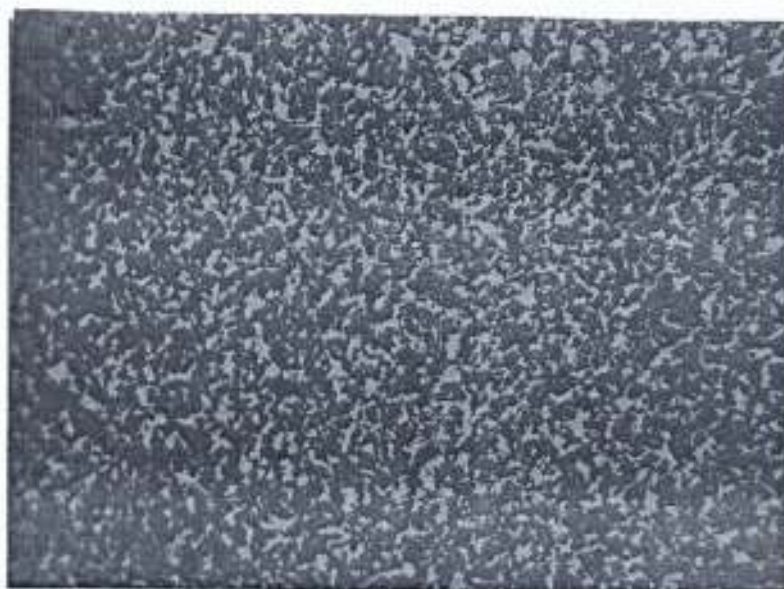
Plate 4.4: Microstructure of Heat Treated Specimen C2 (L+T) (400X) (Duplex ferrite – Martensite Microstructure)
