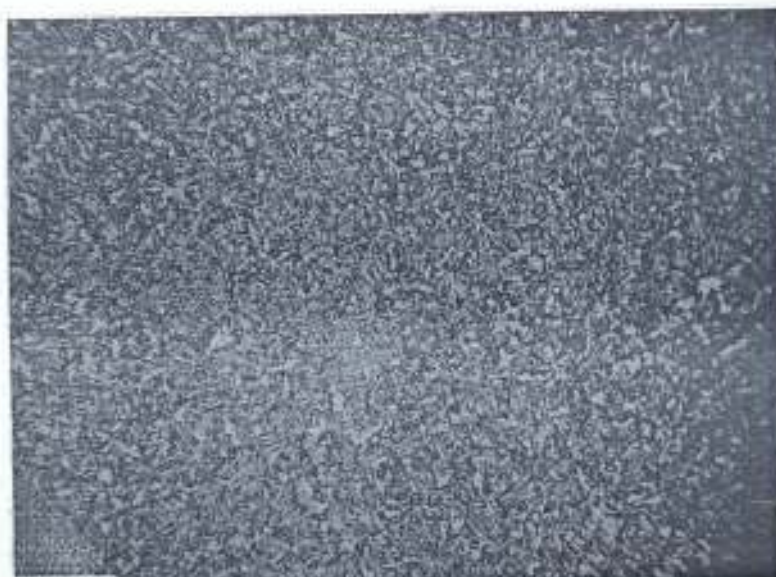
Plate 4.2: Microstructure of Heat Treated Specimen A2 (Q+Q+L+T) (400X) (Duplex Ferrite – Martensite Microstructure)
