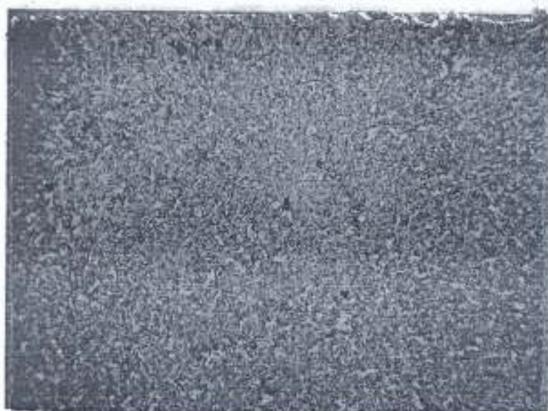
Plate 4.3: Microstructure of Heat Treated Specimen B2 (Q+L+T) (400X) (Duplex ferrite – Martensite Microstructure)
