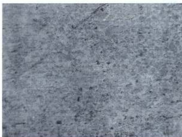
Plate4, 2: Process 1 micrograph of mild steel immersed in 3% KCl solution without inhibitors for 105 days, etched in 2% Nital, showing the effect of corrosion in the microstructure (X160)
