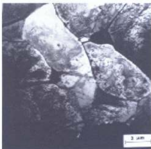
Plate 1AR. Typical TEM microstructure of the as received Al-Mg-Si alloy showing \text{Fe}_3\text{SiAl}_{12} particles, dislocations and few \beta precipitates in a matrix of \alpha -Aluminium rich solid solution.
