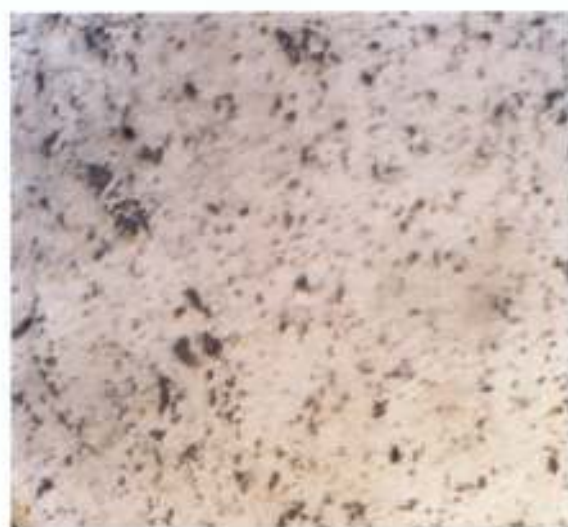
Plate19. Typical microstructure of artificially peak-aged (PA) Al-Mg-Si alloy at 220^{\circ}\text{C} for 6hrs, showing particles of \text{Fe}_3\text{SiAl}_{12} (scriptlike) and precipitates of \text{Mg}_2\text{Si} (small blocky form) in a matrix of Aluminium-rich solid solution. Noted here are relatively smaller forms of the particles of \text{Fe}_3\text{SiAl}_{12} dispersoids. Etched in 0.5 percent HF, 500x.
