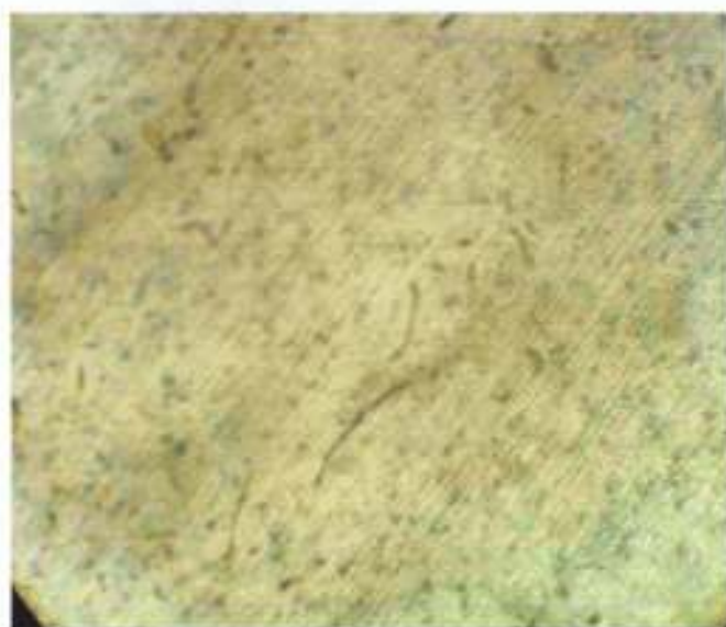
Plate 40 Typical peak aged (PA) microstructure of Al-Mg-Si alloy subjected to TMA IIID processing route showing particles of redistributed \text{Fe}_3\text{SiAl}_{12} (scriptlike), and few precipitates of \text{Mg}_2\text{Si} (lamellar/ small
