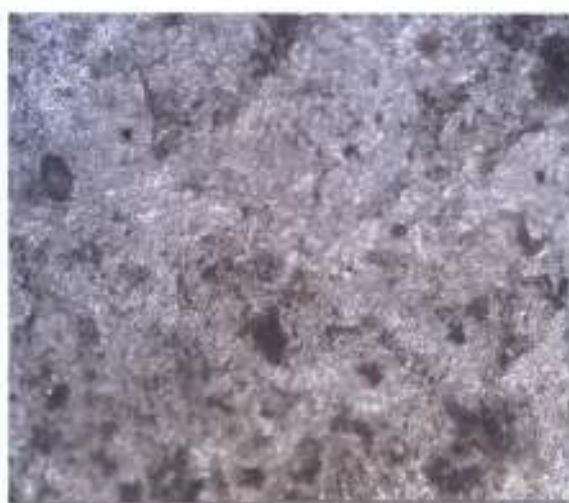
Plate17. Typical microstructure of artificially underaged (UA) Al-Mg-Si alloy at 180^{\circ}\text{C} for 6hrs, showing particles of \text{Fe}_3\text{SiAl}_{12} (scriptlike) and insignificantly few precipitates of \text{Mg}_2\text{Si} (small blocky form) in a matrix of Aluminium-rich solid solution. Noted here are relatively small clusters of the particles of \text{Fe}_3\text{SiAl}_{12} dispersoids. Etched in 0.5 percent HF, 500x.
