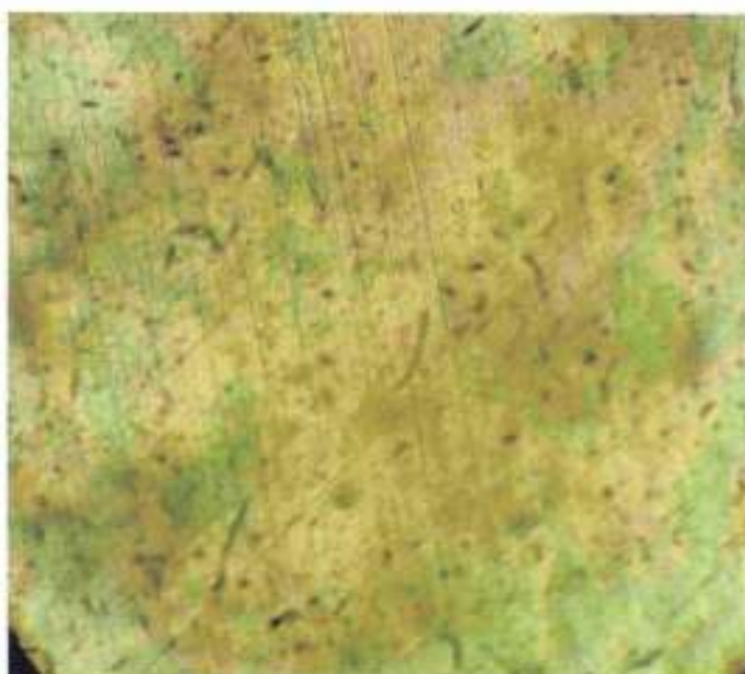
Plate 31 Typical peak aged (PA) microstructure of Al-Mg-Si alloy subjected to TMAIII A processing route showing particles of redistributed \text{Fe}_3\text{SiAl}_{12} (scriptlike), and few precipitates of \text{Mg}_2\text{Si} (lamellar/ small blocky form) in a matrix of Aluminium-rich solid solution . Etched in 0.5 percent HF, 400x.
