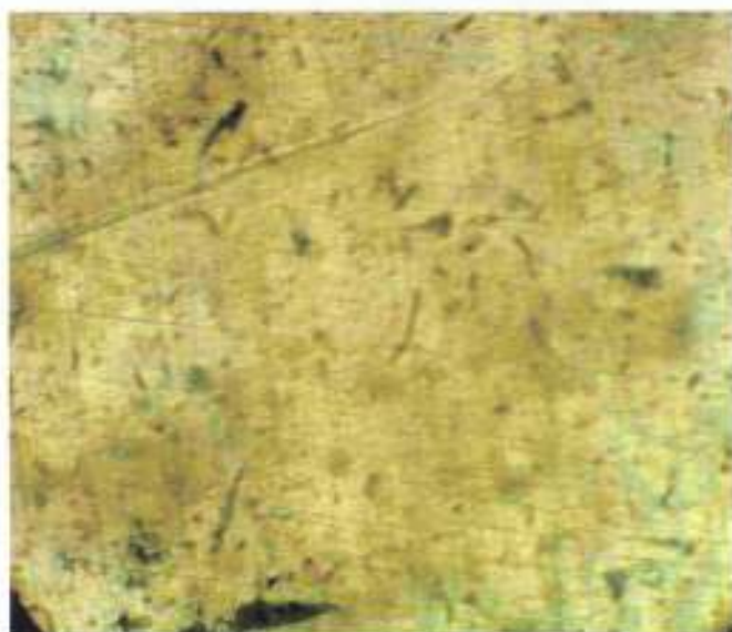
Plate 39 Typical under aged (UA) microstructure of Al-Mg-Si alloy subjected to TMAIIID processing route showing particles of \text{Fe}_3\text{SiAl}_{12} (scriptlike), and few precipitates of \text{Mg}_2\text{Si} (lamellar/ small blocky form) in a matrix of Aluminium-rich solid solution . Etched in 0.5 percent HF,400x
