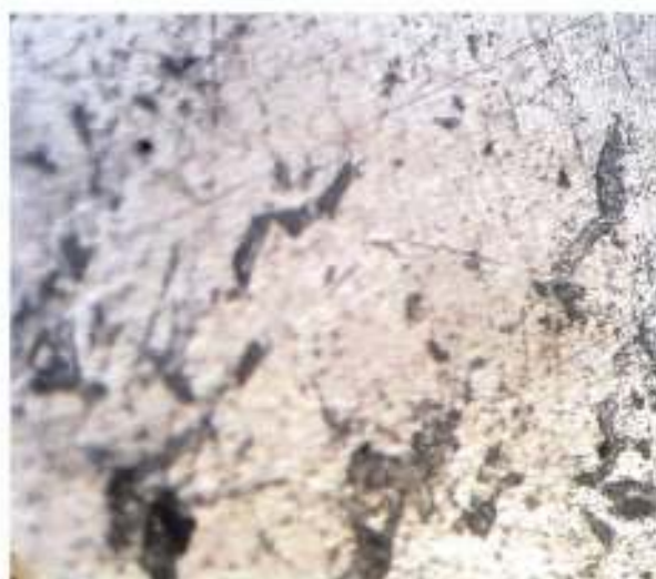
Plate 1. Typical microstructure of Al-Mg-Si alloy; as received (SHT) showing particles of \text{Fe}_3\text{SiAl}_{12} (scriptlike), \text{Al}_5\text{FeSi} (platelike) and \text{Mg}_2\text{Si} (small blocky form) in a matrix of Aluminium-rich solid solution. Etched in 0.5 percent HF, 250x.
