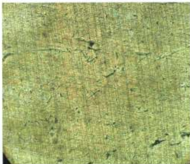
Plate 27 Typical underaged (UA) microstructure of Al-Mg-Si alloy subjected to TMAIID processing route showing particles of \text{Fe}_3\text{SiAl}_{12} (scriptlike), and few precipitates of \text{Mg}_2\text{Si} ( small blocky form) in a matrix of Aluminium-rich solid solution . Etched in 0.5 percent HF, 400x.
