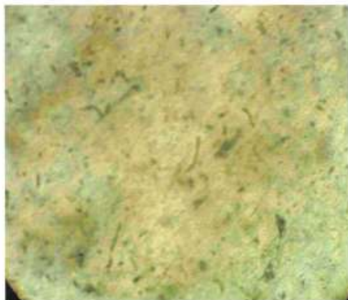
Plate 34 Typical peak aged (PA) microstructure of Al-Mg-Si alloy subjected to TMA IIIB processing route showing particles of \text{Fe}_3\text{SiAl}_{12} (scriptlike), and few
