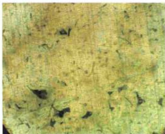
Plate 30 Typical under aged (UA) microstructure of Al-Mg-Si alloy subjected to TMAIII processing route showing particles of \text{Fe}_3\text{SiAl}_{12} (scriptlike) and \text{Mg}_2\text{Si} (lamellar / small blocky form) in a matrix of Aluminium-rich solid solution. A change in the matrix colouration due to a further increase in solute concentration by virtue of 75% preageing is noted here and for all TMAIII processing routes. Etched in 0.5 percent HF, 400x.
