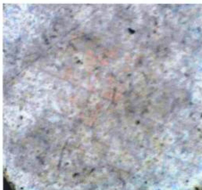
Plate 29 Typical over aged (OA) microstructure of Al-Mg-Si alloy subjected to TMAIID processing route with 20hrs final ageing time, showing particles of \text{Fe}_3\text{SiAl}_{12} (scriptlike), and precipitates of \text{Mg}_2\text{Si} ( lamella/small blocky form) in a matrix of Aluminium-rich solid solution . Etched in 0.5 percent HF, 400x.
