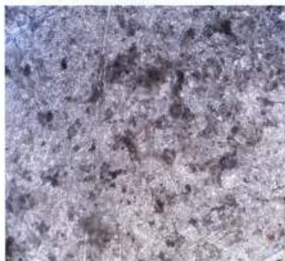
Plate12. Typical microstructure of artificially peak-aged (PA) Al-Mg-Si alloy at 180^{\circ}\text{C} for 12hrs, showing particles of \text{Fe}_3\text{SiAl}_{12} (scriptlike) and scanty precipitates of \text{Mg}_2\text{Si} (small blocky form) in a matrix of Aluminium-rich solid solution. Cells formation is visible. Etched in 0.5 percent HF, 500x.
