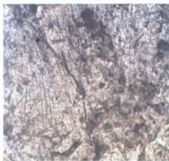
Plate 6. Typical microstructure of Al-Mg-Si alloy; 20% deformation at 240°C, showing particles of Fe 3 SiAl 12 (scriptlike) and Mg 2 Si (lamellar or small blocky form) in a matrix of Aluminium-rich solid solution. Lamellar forms of Mg 2 Si are significantly prominent. Etched in 0.5 percent HF, 400x.
