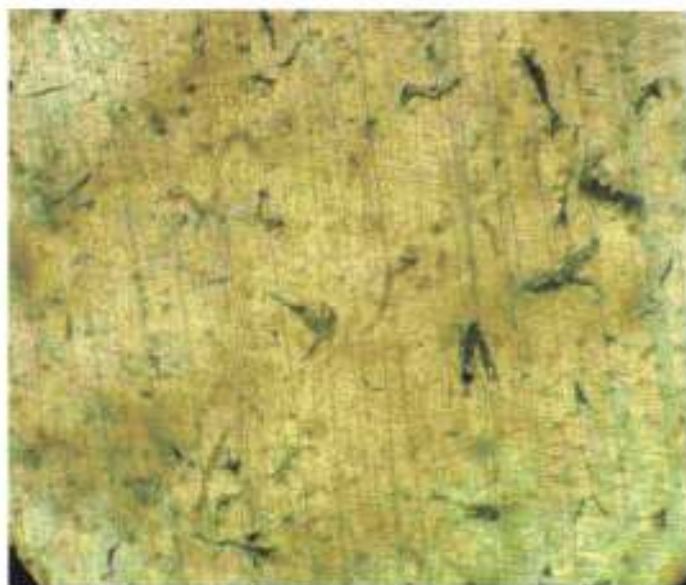
Plate 33 Typical under aged (UA) microstructure of Al-Mg-Si alloy subjected to TMAIIIB processing route showing particles of redistributed \text{Fe}_3\text{SiAl}_{12} (scriptlike), and few precipitates of \text{Mg}_2\text{Si} ( small blocky form) in a matrix of Aluminium-rich solid solution . Etched in 0.5 percent HF,400x
