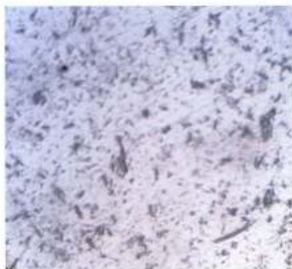
Plate 7. Typical microstructure of Al-Mg-Si alloy; 40% deformation at 240 0 C, showing particles of Fe 3 SiAl 12 (scriptlike) and Mg 2 Si ( small blocky form) in a matrix of Aluminium-rich solid solution. Fewer particles of Mg 2 Si compared to that of Fe 3 SiAl 12 dispersoid. Etched in 0.5 percent HF, 400x.
