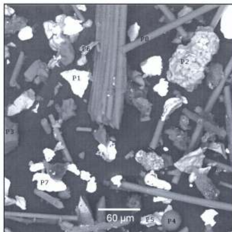
Figure 7.5: Backscattered electron SEM micrograph of dispersed particles of PCB CF P1 – P8 correspond to particles whose EDS spectra are shown in Figure 7.6
