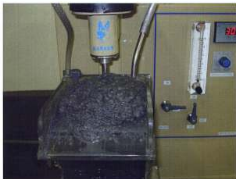
Figure A2.2: Natural hydrophobic froth build up under E21A condition in the first minute of aeration.
