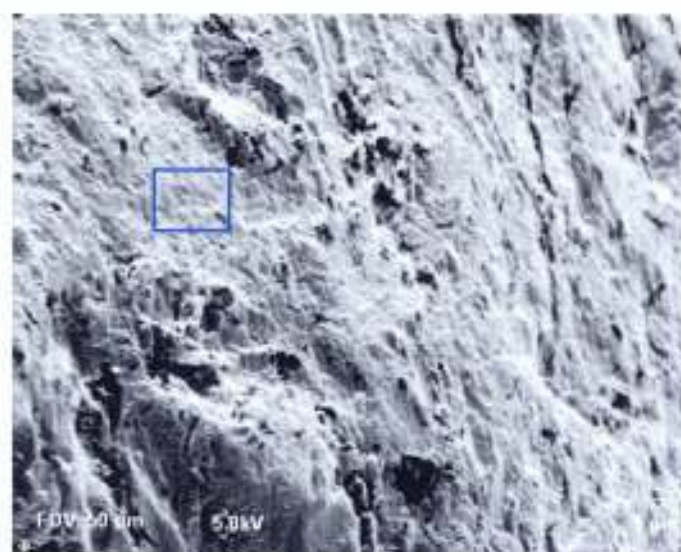
Figure A4.3: SEM secondary electron image on Particle P2 at 5 kV 10 nA primary beam current: Blue square indicates area of analysis.
