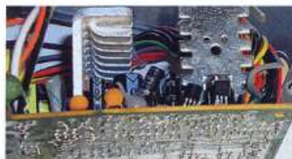
Figure 2.2: Single sided boards
