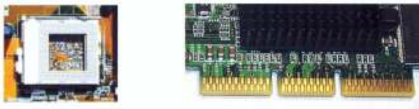
Figure 2.4: ZIF socket (left) and edge connector (right)
