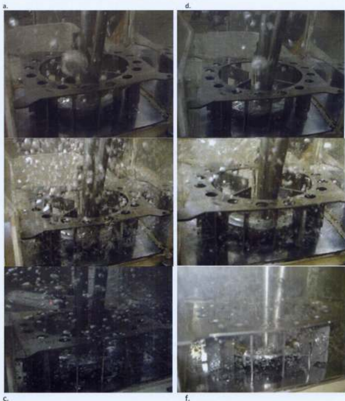
Figure A2.6: Frozen frames showing variation of bubble sizes with impeller speed and aeration rate at: 1000 mlpm aeration and (a) 300 rpm, (b) 400 rpm, (c) 500 rpm; and at 500 mlpm aeration and (d) 300 rpm, (e) 400 rpm, (f) 500 rpm.
