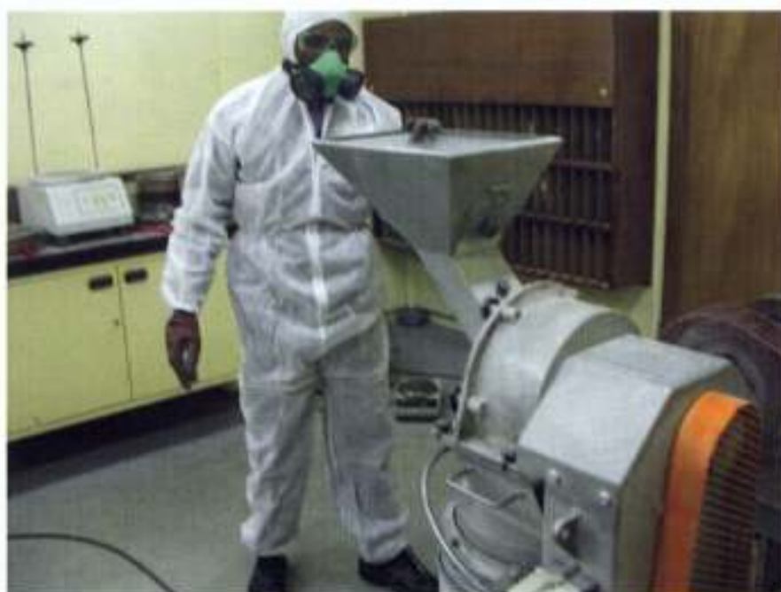
Figure A1.3: Picture showing full PPE gear employed during hammer mill comminution of PCB. The gear includes: N95 respirator, eye shield, laboratory coat and trousers, disposable hooded outer overall, safety shoe and ankle length PVC gloves with fabric inner lining.
