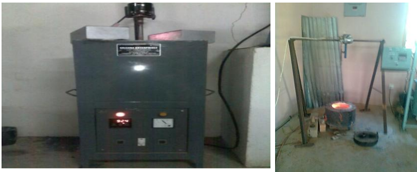
Figure 6. (a) standard automated stir-casting machine, (b) Homegrown stir-casting set-up with innovative mechanical stirring assembly
